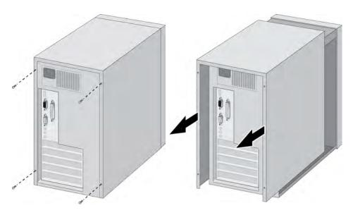
Figure 12. Removing the PC Cover
