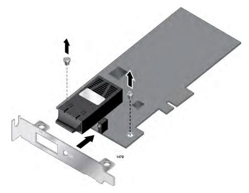
Figure 10. Removing the Low-Profile Bracket
