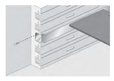
Figure 15. Securing the Adapter Card
