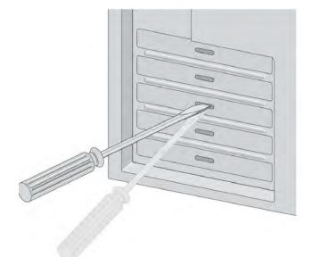
Figure 13. Removing the Faceplate From PCIe Slot
