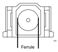
Figure 62. Ferrule in an SC Connector Plug
