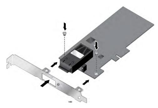
Figure 11. Fastening Screws onto Standard Bracket
