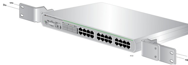
Figure 22. Attaching the Brackets to the Switch
