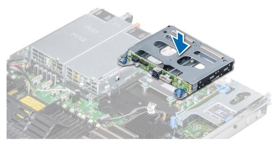
Figure 97. Installing the rear drive cage
