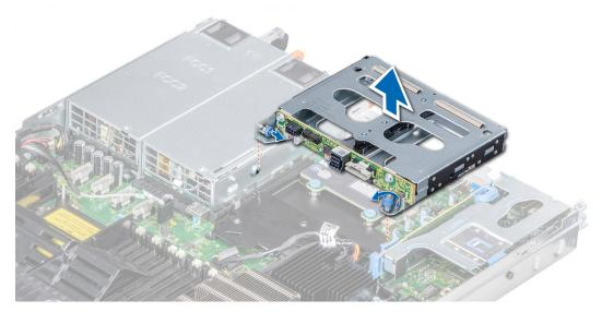
Figure 96. Removing the rear drive cage
