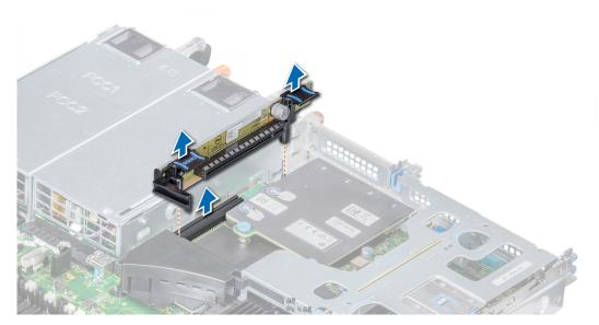
Figure 53. Removing the expansion riser 2A
