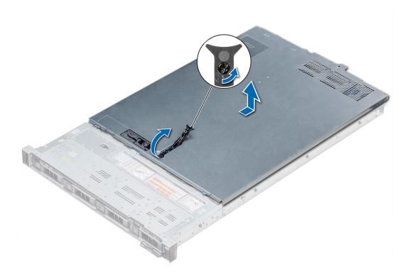
Figure 22. Removing the system cover
