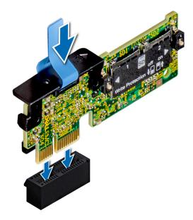
Figure 71. Installing optional IDSDM module
