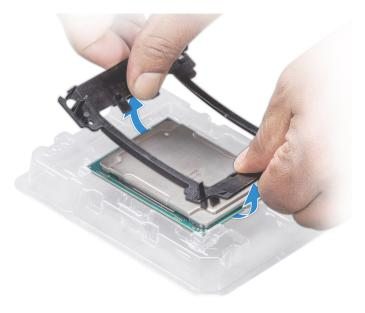
Figure 46. Removing the processor bracket
