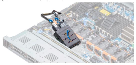
Figure 42. Removing the NVDIMM-N battery
