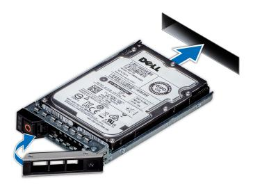
Figure 27. Installing a drive carrier
