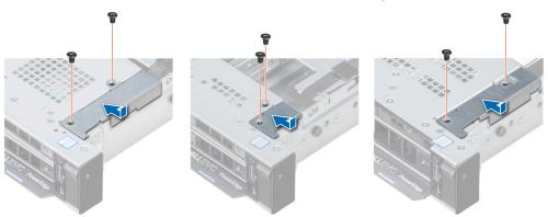
Figure 120. Installing the cable cover
