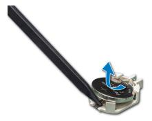
Figure 98. Removing the system battery
