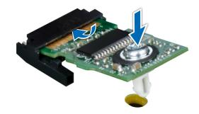
Figure 112. Installing the TPM
