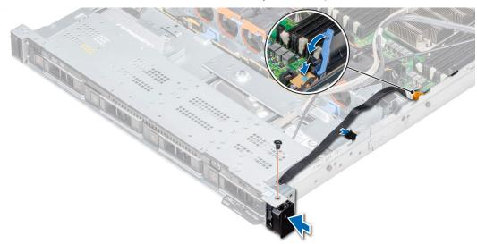
Figure 119. Installing the right control panel
