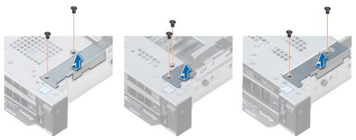
Figure 117. Removing the cable cover
