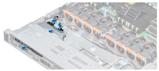
Figure 104. Removing optical drive
