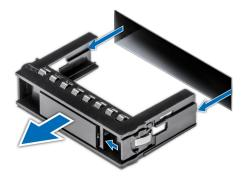
Figure 24. Removing a drive blank
