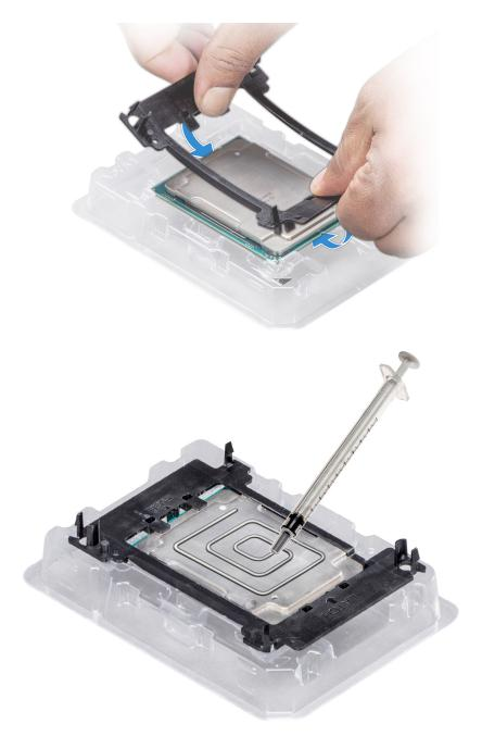
Figure 48. Applying thermal grease on top of the processor
