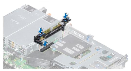
Figure 57. Installing the expansion riser 2A
