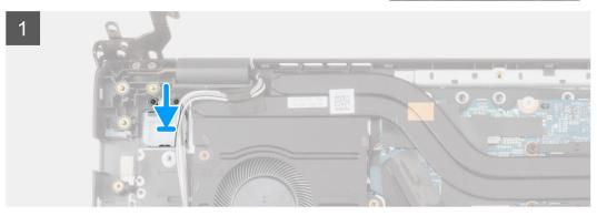
Align and place the power-button board into the slot on the palmrest assembly.
