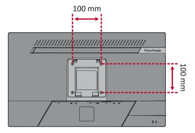
**6.** Follow the instructions that come with the wall mounting kit to mount the monitor onto the wall.
