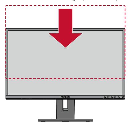
**NOTE:** When adjusting, press down firmly along the adjustment track.
