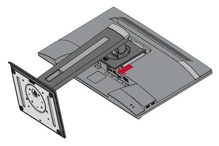
**5.** Attach the mounting bracket to the VESA mounting holes at the rear of the device. Then secure it with four (4) screws (M4 x 10 mm).
