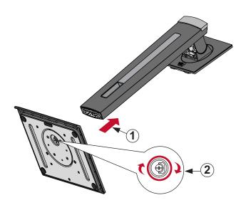
**4.** Align and slide the upper hooks of the monitor stand into the stand mounting slots as shown in the illustration below:
