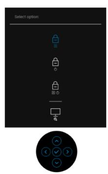
**3.** Move the joystick to highlight the Diagnostic icon and then press the joystick to confirm. A gray test pattern appears.
