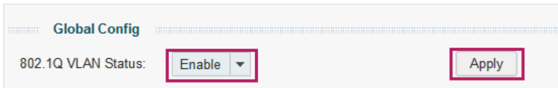
Figure 5-2 Configuring 802.1Q VLAN
